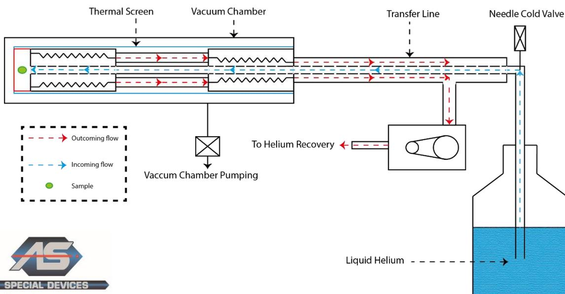
The cooling power of the cryostat is a function of the Helium flow rate and the capacity of the exchangers to transfer heat (efficiency). This power is determined by two factors: firstly by the cold valve on the transfer tube, which limits the Helium flow rate, and secondly by the pumping speed of the Helium vacuum pump.
