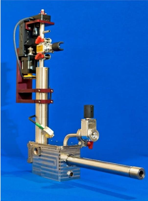
This instrument allows a quick sample change, we are talking minutes, and an accurate sample positioning. The sample chamber works with a Helium gas flow assuring a good thermalization and a precise temperature measurement of the sample. Particularly useful for low thermal conductivity samples, its sample holder can accommodate 4 pellets of 5mm diameter.
